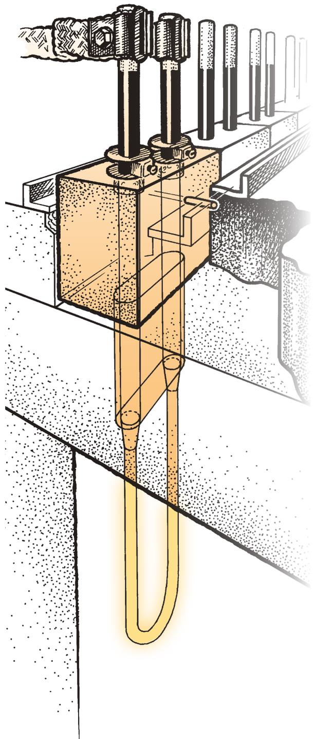
Fig. 9 Kanthal Super elements in ceramic fiber lined furnaces.
