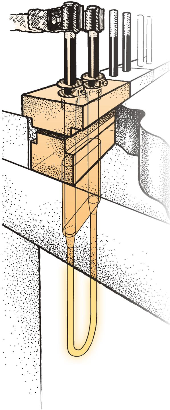
Fig. 8 Kanthal Super elements in ceramic fiber lined furnaces.
