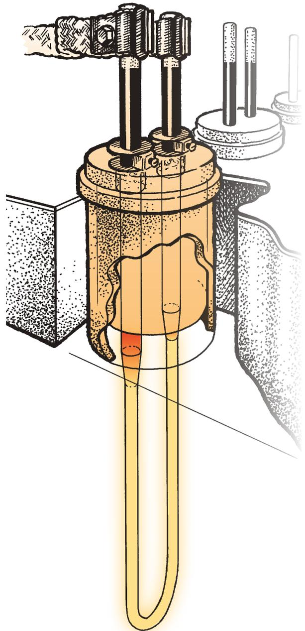
Fig. 5 Kanthal Super elements in ceramic fiber lined furnaces. The passage plugs with a flange are made of ceramic fiber and fitted into ceramic fiber sleeves.
