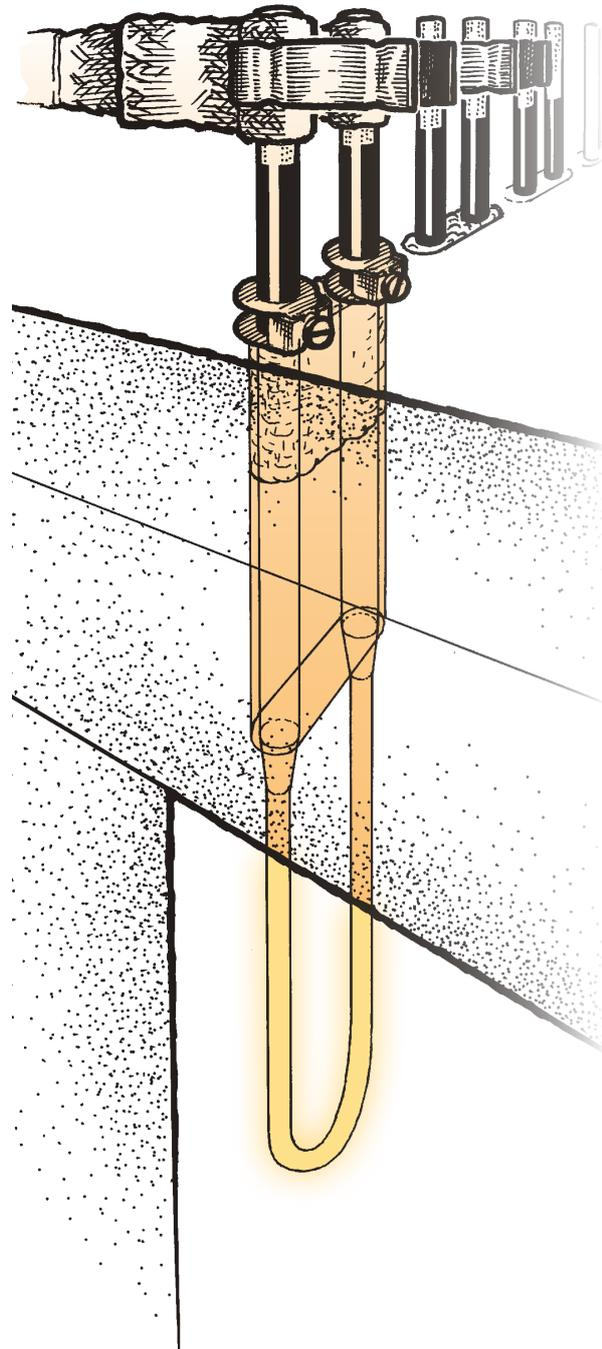
Fig. 7 Kanthal Super elements in ceramic fiber lined furnaces installed through oval slots in the roof.
